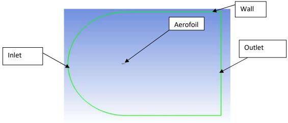
Figure 1. The geometry and Flow domain
