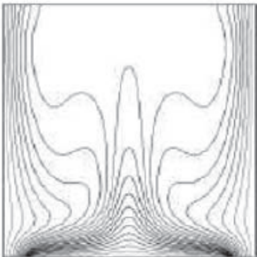
Fig 6.3: temperature contour for Ra of order 10^5
