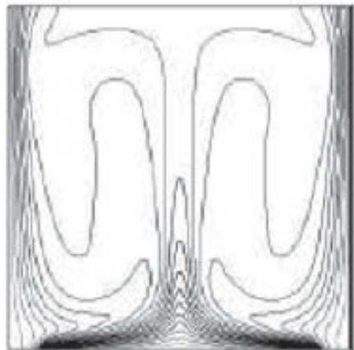
Fig 6.4: temperature contour for Ra of order 10^6
