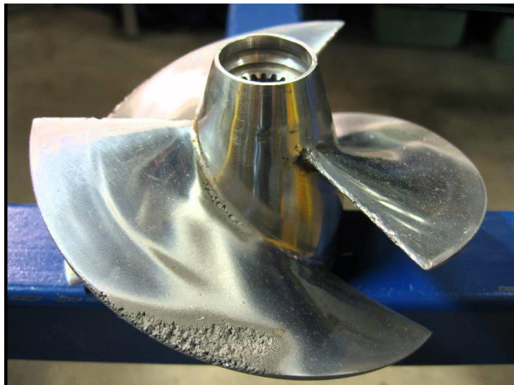
Submarine propeller Cavitation (source: Wikipedia)
