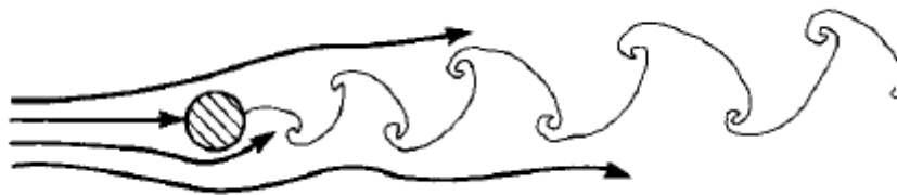
Figure 2. Re = 140 flow across a cylinder [1].
