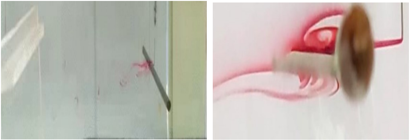
Figure 3.5: Experimental Visualization Of Flow Over Cylinder With & Without Rigid Splitter Plate @ Re=50 – Additional Results (Only Experimental) To Observe The Re-Circulation Zone Formed
